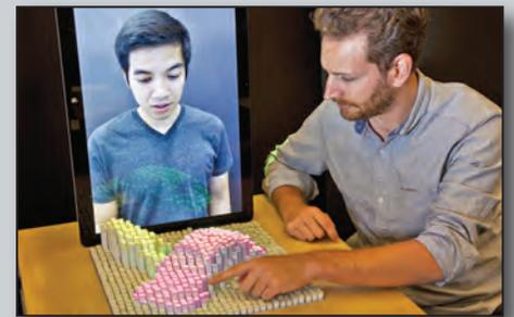
Figure 2. Physical Telepresence provides physical embodiment, remote manipulation and new capabilities through computer-mediated teleoperation. Here, local and remote users physically interact with a 3D car model.
